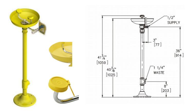
Model S0320 is our free standing eye wash with plastic bowl. Complete with plastic eye/face spray heads, an inline stainer and stay-open 1/2" ball valve with a push handle operation. Complete with cast iron floor flange to securely bolt the unit to the floor.
